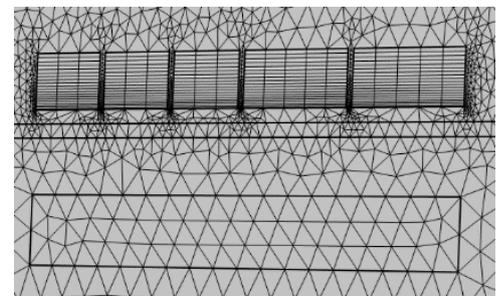
Fig. 7. Mesh on the radial cross section of stator core
