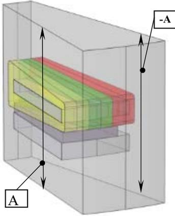
**Fig. 3.** Modelling domain for solving the magnetostatic boundary value problem, boundaries with antiperiodic conditions
