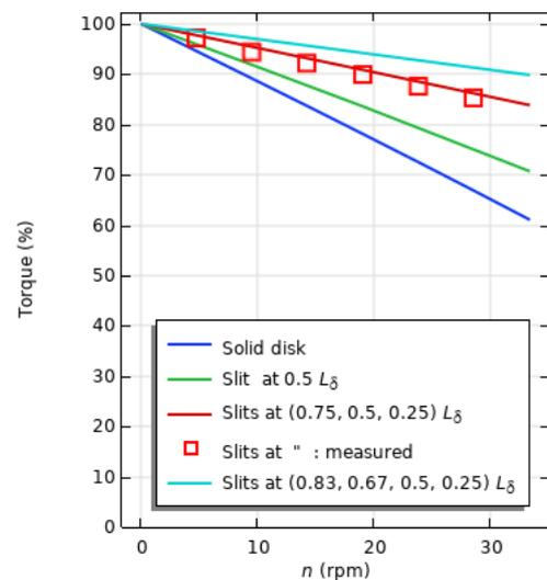
**Fig. 9.** Torque versus rotational speed
