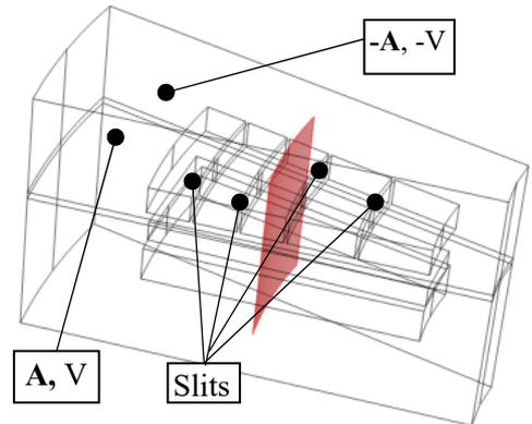
Fig. 5. Domain for simulation of eddy current losses in stator core and central cross section of magnetic core
