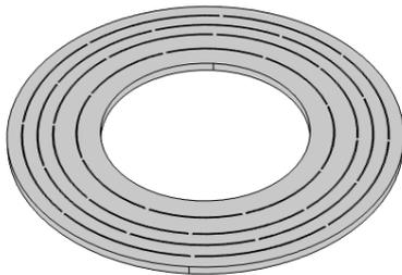
Fig. 2. Stator core with four slits
