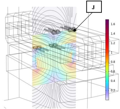
**Fig. 4.** Magnetic flux density (norm) in the middle cross section and current flow in phases  $A, C$
