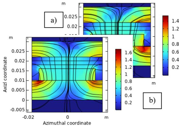
**Fig. 8.** Norm and streamlines of magnetic flux density (T); a) without slits; b) four slits
