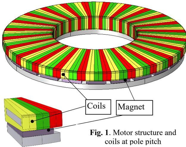
Fig. 1. Motor structure and coils at pole pitch
