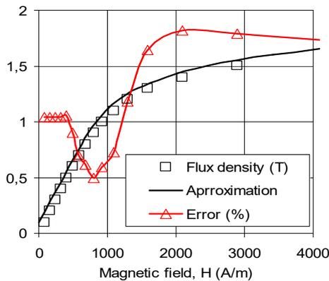
Fig. 6. Magnetization curve and approximation error
