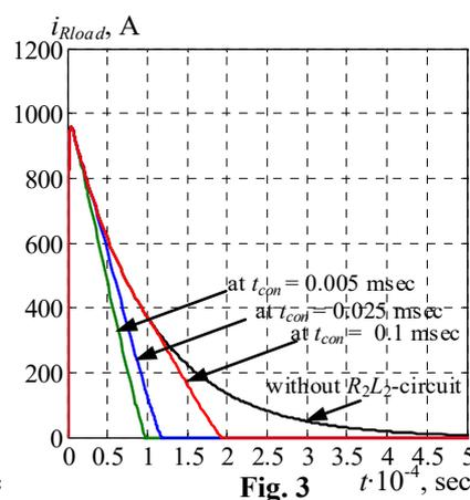
reduces the discharge time by 7.2 (6 and 3.6) times, respectively, compared to the mode without connecting. In this case, the average pulse power in the load increases 4.6 (4.5 and 3.5) times, respectively.
